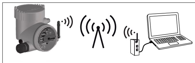
Fig. 41: Transmission of measured values and remote parameter adjustment of the sensor via mobile phone network.
